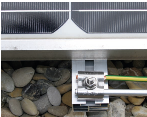
Figure 3 UNI earthing clamp: A stainless steel intermediate element prevents contact corrosion, thus establishing reliable long-term connections between different conductor materials
