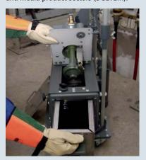
After lifting the conveying pump out of the HT mass, the oil reservoir can be removed from the NFG MS for refilling.
