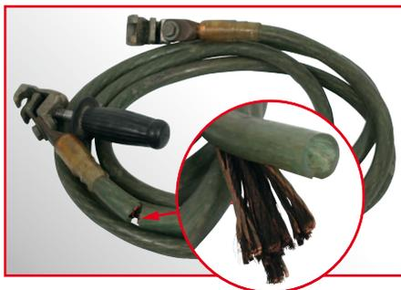
Faulty earthing and short-circuiting device, short-circuiting cable with advanced black colouration
