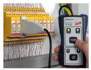
Figure 8.2.6.2 LifeCheck arrester testing by means of DRC LC M1+
