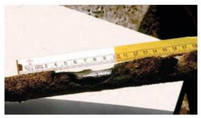
Figure 5.9.6 Corrosion of a galvanised earth rod after 7 years
