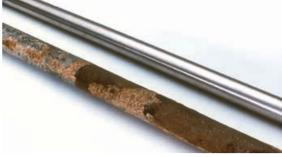
Figure 5.9.7 Corrosion of a galvanised earth rod (below) and a stainless steel earth electrode (above) after 2.5 years
