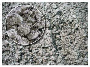
Figure 5.5.2.27 Fresh concrete with steel fibres
