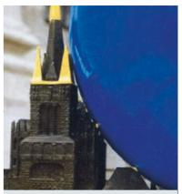
A rolling sphere cannot only touch the steeple, but also the nave of the church at multiple points, as this model experiment shows. All these points are potential points of strike.
