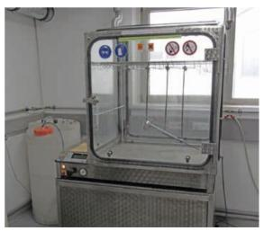
Figure 5.8.2 Test in a Kesternich chamber
