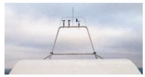
Figure 5.1.10.2 Lightning protection for the anemometers of a wind turbine
