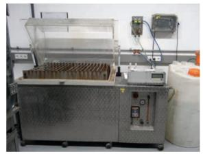
Figure 5.8.1 Test in a salt mist chamber
