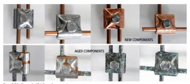
Figure 5.8.3 New and artificially aged components
