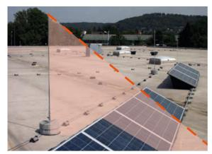
Figure 9.18.14 Determination of the protected volume using the protective angle method
