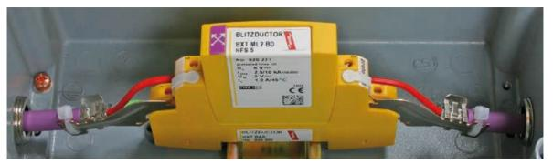
Figure 6.3.3 EMC spring terminals for the protected and unprotected side of a BLITZDUCTOR XT for permanent low-impedance shield contact with a shielded signal line; with snap-on insulating cap for indirect shield earthing, cable ties and insulating strips.
