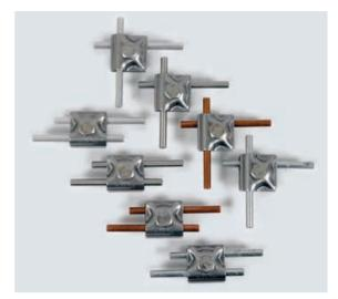
Figure 5.8.4 Test combinations for MV clamps (parallel and cross arrangement)
