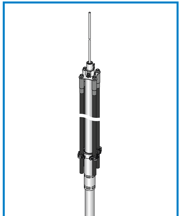
Figure 9 HVI®long Conductor installed outside the supporting tube - Complete
