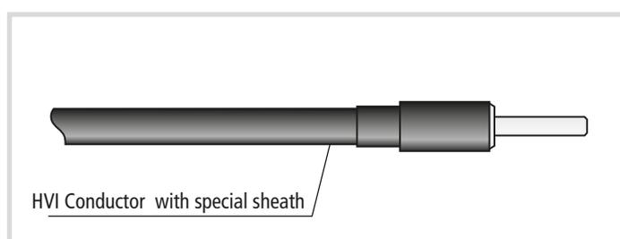
**Figure 4f** HVI® Conductor I pre-assembled or HVI® long Conductor I
