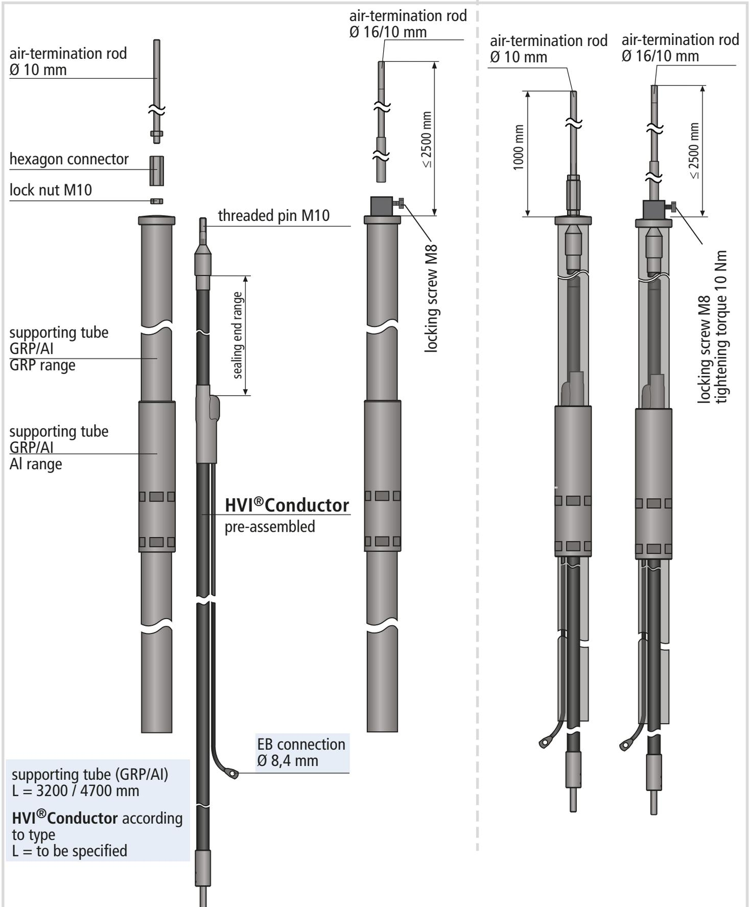
**Figure 9** HVI® Conductor pre-assembled - Integrated in supporting tube
