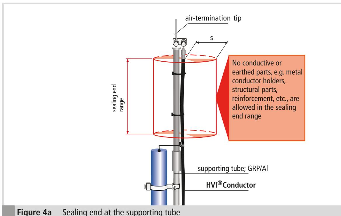
**Figure 4a** Sealing end at the supporting tube
