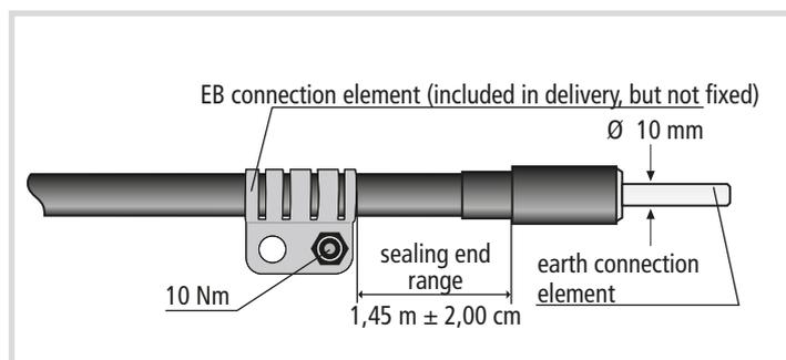
**Figure 4d** HVI® Conductor II and III pre-assembled or HVI® long-Conductor II and III
