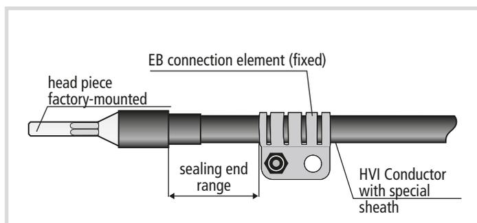
**Figure 4c** HVI® Conductor I, II and III pre-assembled
