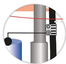
**connection to the equipotential bonding of the building**
