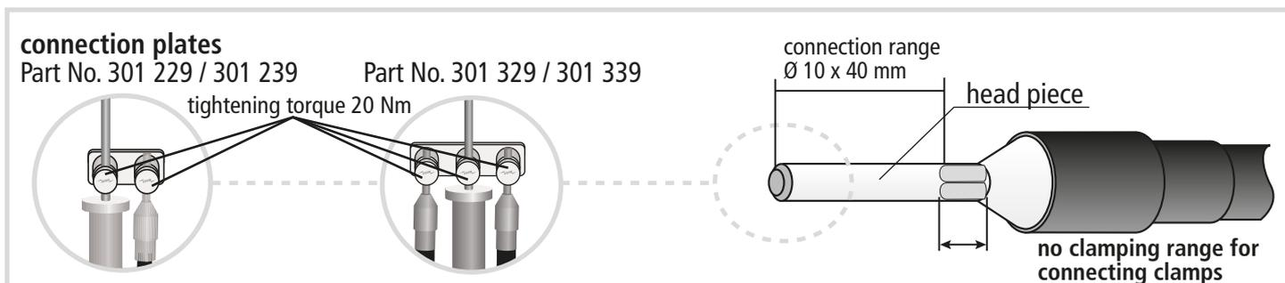
**Figure 8** Connection possibilities / Head piece (details of Figures 3 and 14)
