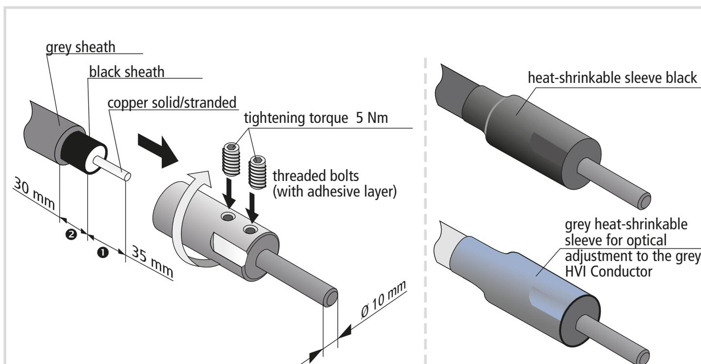
**Figure 5** Mounting of the earth connection element / connection element
