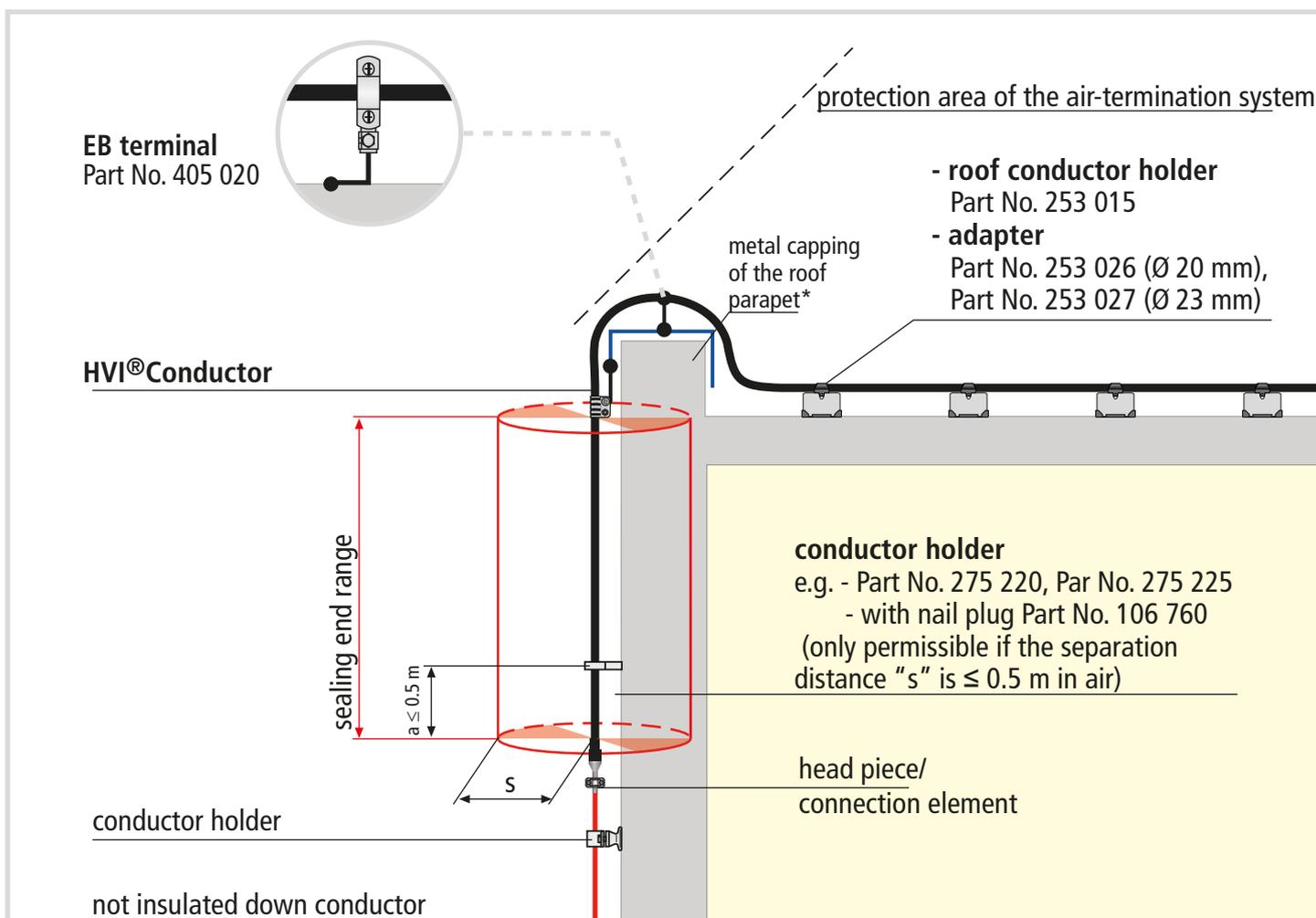
**Figure 7** Transition **HVI® Conductor** to bare down conductor;
