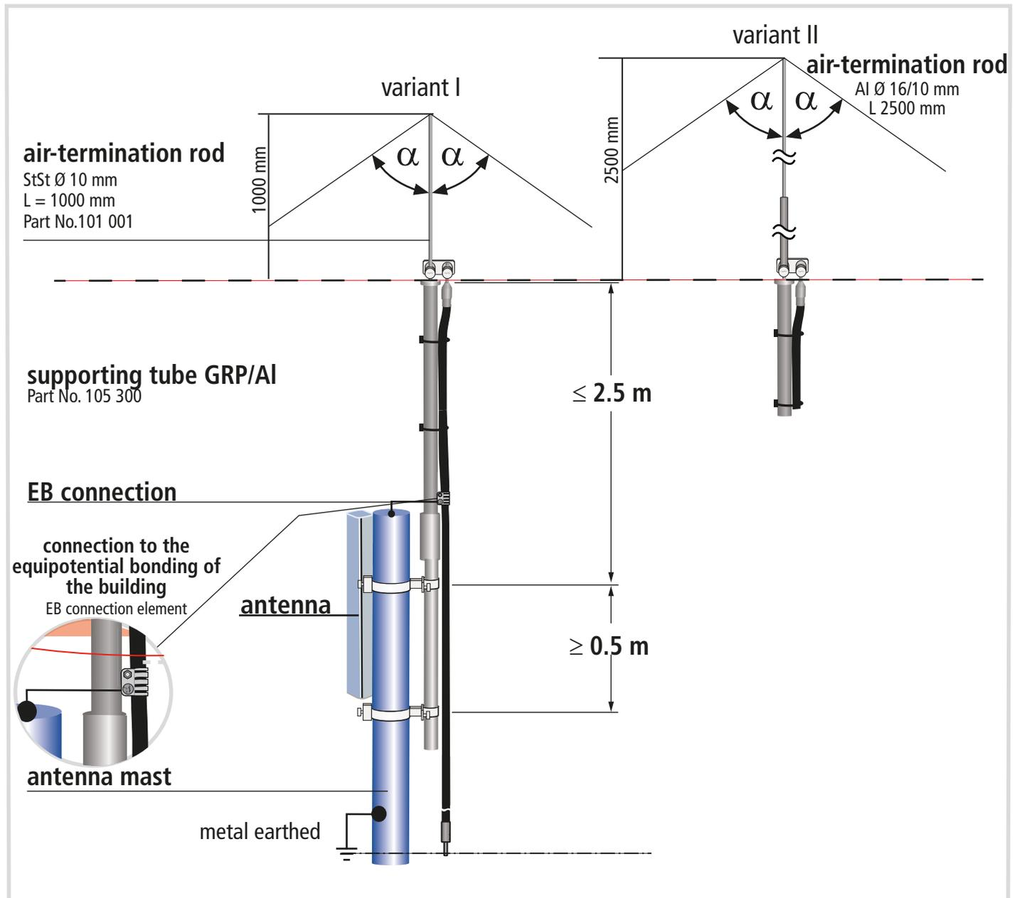
**Figure 12** Supporting tube for a max. wind speed of 185 km/h (variant I)
