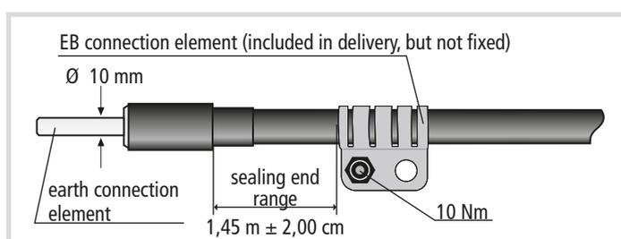
**Figure 4e** HVI® long Conductor I, II and III
