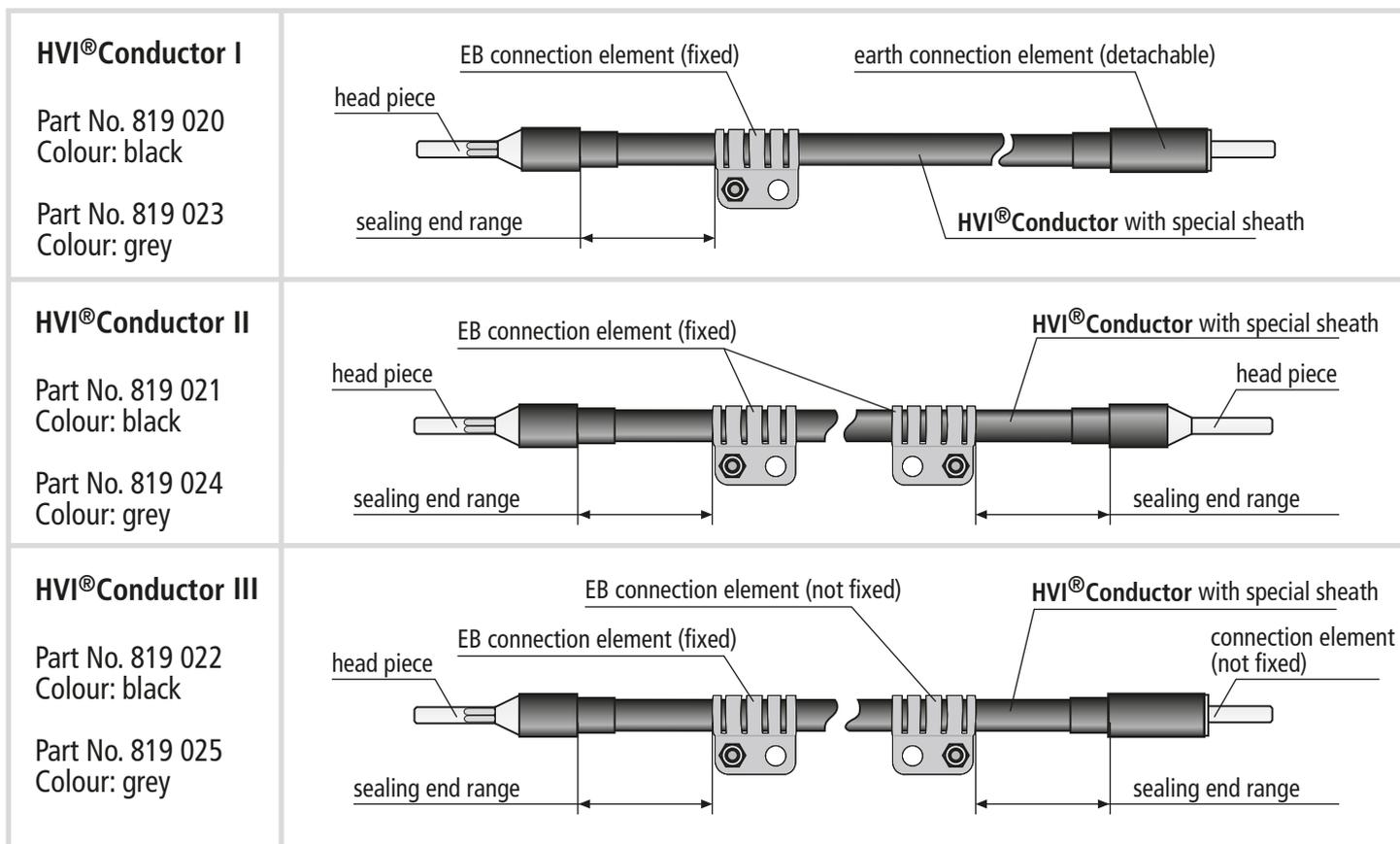
**Figure 1** Design of the HVI® Conductor as assembled conductor with factory-mounted head piece
