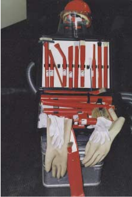
Figure 2: Cleaning set for low-voltage installations with personal protective equipment
