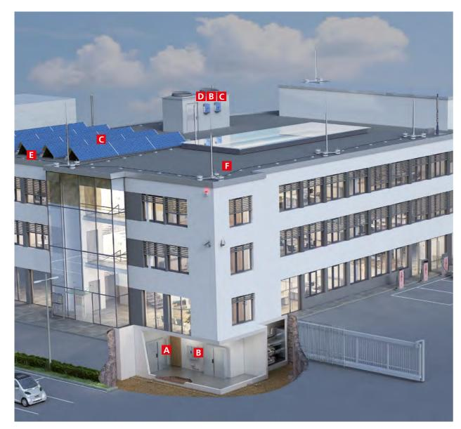
The PV modules must be located in the protected volume of the isolated air-termination system – whilst also maintaining the separation distance "s".
