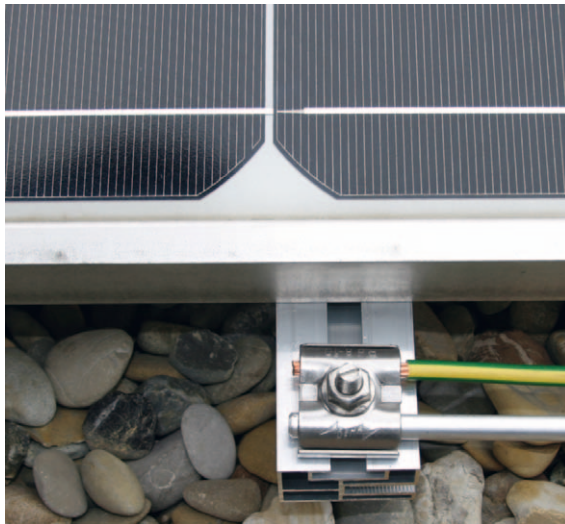
Figure 1 UNI earthing clamp: A stainless steel intermediate element prevents contact corrosion, thus establishing reliable long-term connections between different conductor materials.
